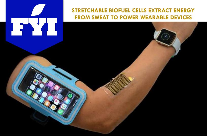
A team of engineers has developed stretchable fuel cells that extract energy from sweat and are capable of powering electronics, such as LEDs and Bluetooth radios. The biofuel cells generate 10 times more power per surface area than any existing wearable biofuel cells. The devices could be used to power a range of wearable devices.
